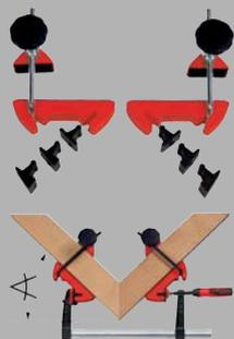
$\sphericalangle = 22,5^\circ / 30^\circ / 45^\circ / 60^\circ$
