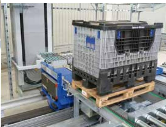
By employing an advanced, contactless current and data transmission technology, the **SpeedPorter** vehicle operates extremely quiet and this for speeds up to 2.5m/s!
